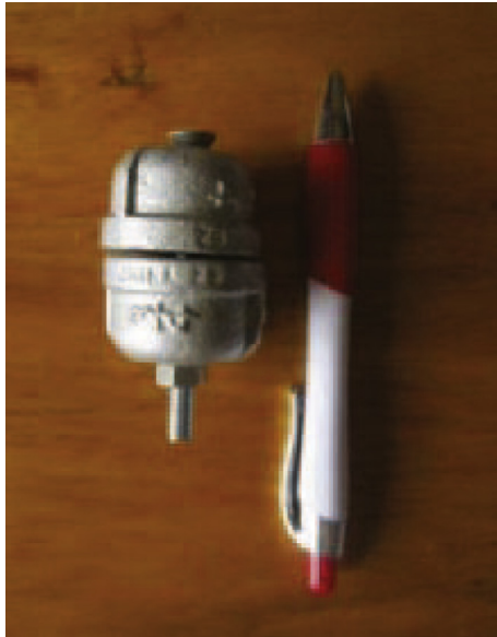
Fig. 4 – SUM holder designed to encase the stove use monitor to protect it from malfunctions when exceeding temperatures of 85 °C.
