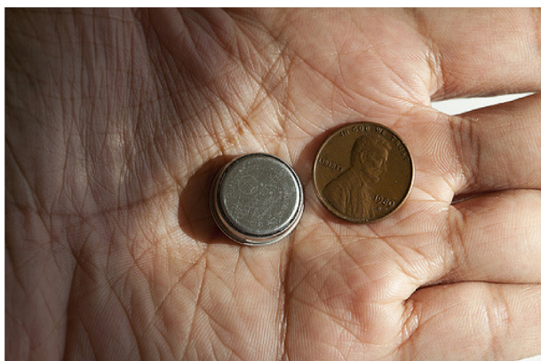
Fig. 1 – Photograph of stove use monitoring system (SUMs).
